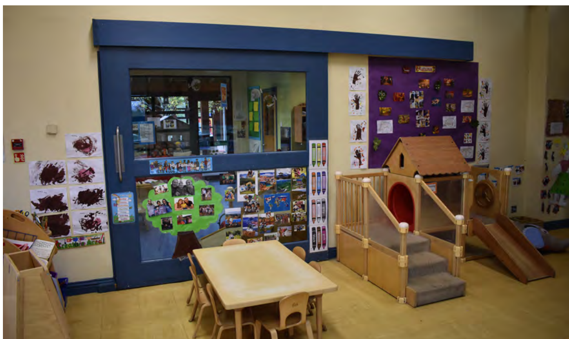
Figure 46. Large sliding door providing the flexibility to open up or close off spaces. Tigers Childcare, Blanchardstown, Dublin 15.
